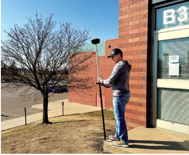
A GNSS+IMU+CAMERA INTEGRATION: The Tersus Trek is being used on a survey for a school expansion project.
