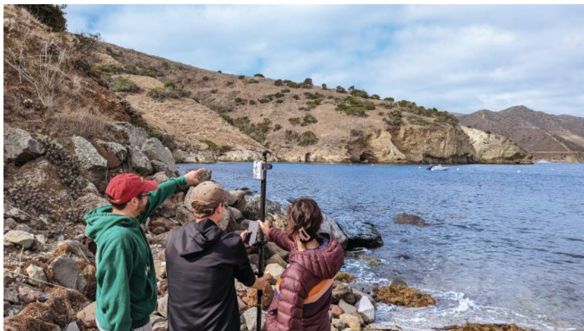
USC SSI GIST graduate students collect field data with the Eos Arrow 100 submeter GNSS receiver during the field excursion week of the Spatial Data Acquisition course in the fall of 2022.
