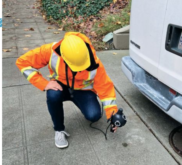
FOR ITS HANDHELD, camera-based 3D mapping system, Looq AI opted for a high-precision GNSS board from Septentrio to integrate with an IMU for their automated PPK and AI-processed workflow.
